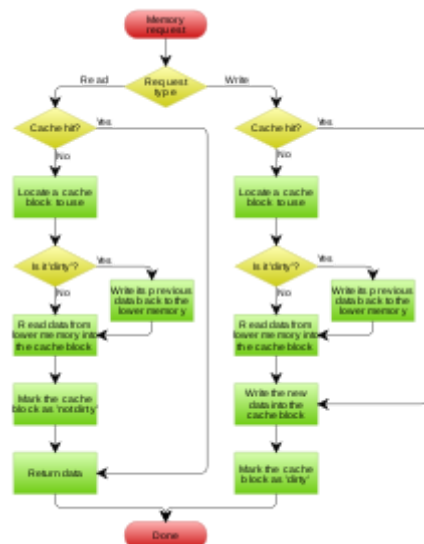
A write-back cache with write allocation
