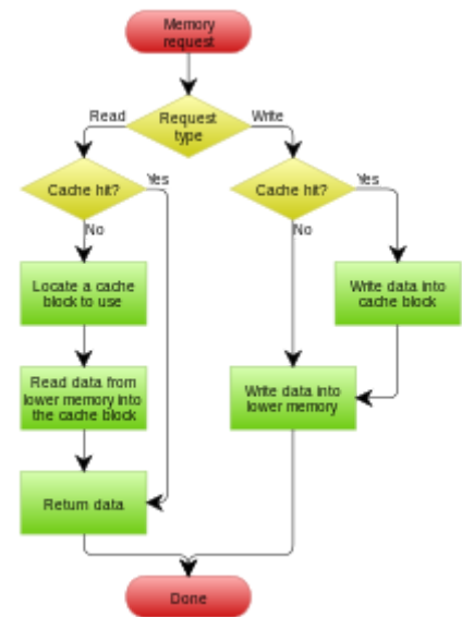
A write-through cache with no-write allocation
