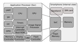
Figure 1: The basic design of a modern smartphone.
