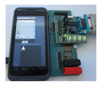
Figure 5: This is one of our Aava devices. It runs a VM with Android and another VM hosts standard Linux. A debug board is attached to the right, which provides a serial line.
